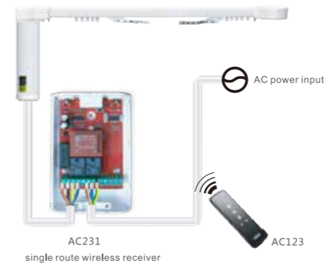
Wiring diagram for AC line switching curtain motors (AM70-1/100-EQ-QP/AM70-2/80-EM-QP)
